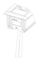
Fixed Power Supply Cable through the bottom of the profile
